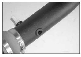
20. After marking the intake tube, remove from vehicle and drill a 7/8" hole into the intake tube then install the provided grommet as shown.
