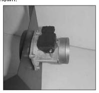
11. Assemble the mass air adapter, heat shield, gaskets and the mass air sensor using the hardware provided.
