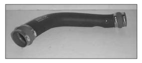
16. Secure the provided hump hoses onto the K&N<sup>®</sup> intake tube as shown using the provided hose clamp.
