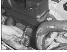
5) Loosen and remove the two nuts that secure the resonator.
