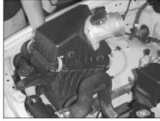
4. Loosen the three bolts that secure the air cleaner
