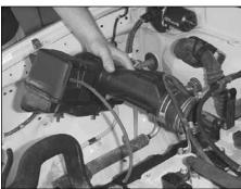
7. Loosen the hose clamp at the throttle body and remove the remaining section of the intake assembly.
