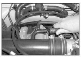
6. Vehicles equipped with an idle air vent line, disconnect vent line as shown.
