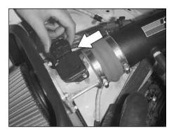
27. Reconnect the mass air sensor electrical connection.
