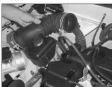
3. Loosen the two hose clamps on the intake hose and remove the intake hose as shown.
