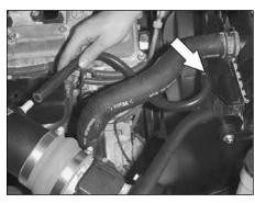
25. Install the provided silicone hose onto the EVAP canister vent and secure the other end onto the  $K\&N^{\otimes}$  intake tube as shown.
