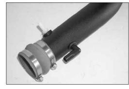
21. Install the 90 degree fitting into the intake tube as shown.
