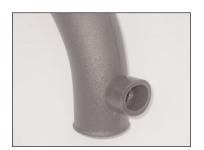
8c. Install the resonator grommet provided into the 1-3/8" hole drilled in step #8 as shown. **NOTE: Be sure to remove any burrs in the hole after drilling.**
