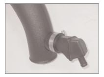
8d. Install the crank case vent resonator into the grommet installed in step #8c and secure with the provided hose clamp.
