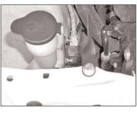
13. Install the twist bracket onto the existing air box-mounting hole with the provided hardware as shown. Do not tighten completely.
