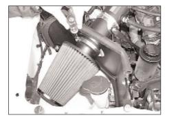
22. Install the K&N<sup>®</sup> air filter onto the K&N<sup>®</sup> intake tube and secure it with the provided hose clamp. NOTE: Drycharger® air filter wrap; part # RC-4700DK is available to purchase separately.
