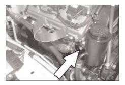
16a. On 2003 and later vehicles, install the saddle bracket assembly onto the motor using the bolt from step 15c. Do not tighten completely.
