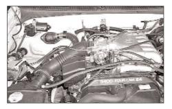
3. Disconnect the three hoses from the air box resonator and intake hose. NOTE: Some 03 models may only come equipped with two vent lines.
