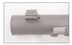
9. Install the mass air sensor into the K&N<sup>®</sup> intake tube using screws and spacers provided.
