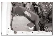
17. Install the heat shield and secure it to the new  $K\&N^{\textcircled{R}}$  brackets with the hardware provided as shown. Do not tighten completely.
