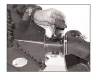
7. Loosen and remove the screws that secure the mass air sensor, then remove the mass air sensor.
