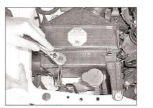
5. Loosen the three bolts that retain the air box assembly.
