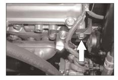
15c. On 2003 models, remove the bolt from power steering bracket as shown
