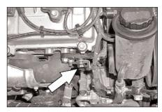
15. On 1999-2002 vehicles loosen and remove the bolt that secures the wire harness bracket located directly behind the power steering reservoir.
