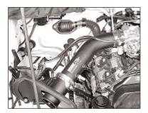
19. Install the K&N<sup>®</sup> intake tube onto the throttle body, and then tighten the hose clamps at the throttle body and saddle bracket.
