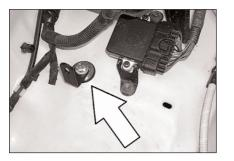
12. Install the "L" bracket onto the existing air box-mounting hole. **NOTE: Rubber washer & fender washer should be mounted between the fender and the bracket.** Do not tighten completely. 15b. On 2003 and later models, remove wire harness from bracket then turn bracket over and mount to engine as shown, then re-install wire harness.
