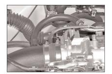
21. On 1999-00 models, attach the provided silicone hose onto the crankcase vent and connect it to the K&N^ $^{(\!8\!)}$  intake as shown.
