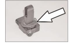
8. Apply the provided gasket to the mass air sensor, with the sticky side down.
