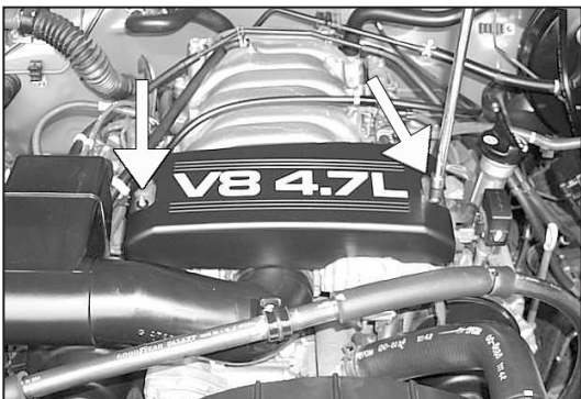
3. Loosen and remove the acorn nuts that secure the throttle body cover, then remove the cover.
