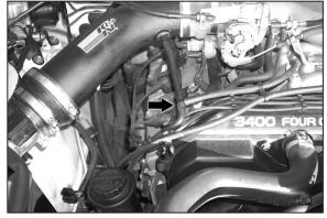
20. Install the rubber hose and vacuum "T" as shown.
