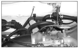
21. Remove the stock crankcase vent hose and replace it with the provided silicone hose and hose clamp. Secure it to the vent on the K&N<sup>®</sup> intake tube.
