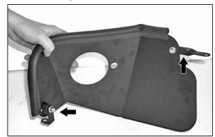
10. Install the two brackets onto the heat shield as shown.
