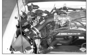
26. Reconnect the vehicle's negative battery cable. Double check to make sure everything is tight and properly positioned before starting the vehicle.
