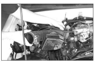
4. Unhook the wire harness from the factory intake tube, then loosen the hose clamps on the intake tube. Remove the factory intake tube as shown.
