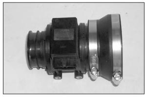
14. Install the plastisol adapter and hose clamps onto the mass air sensor as shown.
