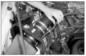
24. On vehicles equipped with a EVAP vent line attached to the airbox, connect the factory EVAP line to the hose mender/vent line installed into the K&N<sup>®</sup> air filter during step #22.
