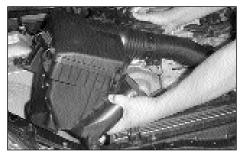
9. Remove the complete air box assembly. NOTE: K&N Engineering, Inc., recommends that customers do not discard factory air intake.
