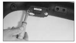
13. Install the provided bushings into the mass air sensor as shown.
