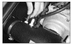
24. Install the stock vacuum line onto the new air intake tube.
