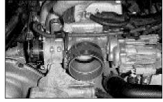
21. Install the silicone hose onto the throttle body.
