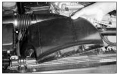
7. Loosen and remove the bolts which holds the fresh air intake, then remove intake.
