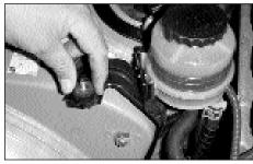
19. Install the rubber studs to the stock air box mounting location as shown.
