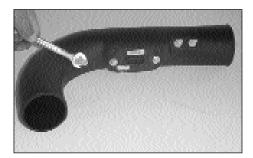
15. Install the barbed vents into the air intake tube
