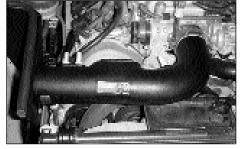
22. Install the new air intake tube to the throttle body and heat shield then tighten the hose clamps.
