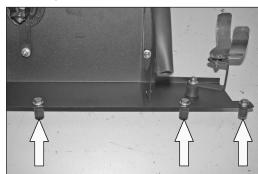
15. Install the inserted nuts onto the heat shield using the provided hardware.
