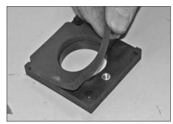
24. Install the supplied gasket onto the mass air adapter plate as shown.
