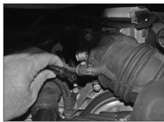
3. On "TIPTRONIC" equipped vehicles with a vent line connected to the stock intake tube next to the throttle body, loosen the hose clamp that secures the vent line and disconnect the vent line from the intake tube.
