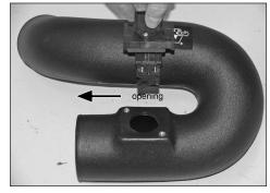
26. Install the mass air sensor assembly into the K&N® intake tube as shown and secure with the provided hardware.
