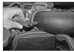
29. On "TIPTRONIC" equipped vehicles, install the 90° vent fitting assembled in step #28 onto the vent line and align it with the K&N® intake tube for best fit, place a mark on the tube for a drill location.
