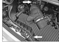
4. Loosen the hose clamp, which secure intake tube to the throttle body, and remove the air box mounting bolt shown.
