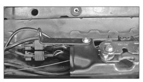
16d. Install the "L" bracket (010040) onto the hood latch support and secure with the provided hardware as shown.
