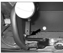
16a. Align the "L" bracket (010040) with the heat shield and secure with the provided hardware as shown.
