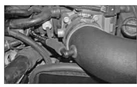
31. Install the 90° hose mender into the grommet installed in step #30 as shown.
