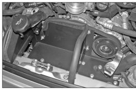
16e. Reinstall the heat shield assembly and secure with the provided inserted nuts and "L" bracket (070066). Secure the "L" bracket to body with the provided hardware.
