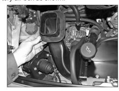
18. Install the fresh air supply duct into the heat shield and align duct so that it lines up with the bellows on the hood and with the heat shield as shown.
