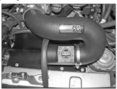
27. Install the K&N® intake tube onto the throttle body and saddle clamp, secure with the provided hose clamps.
