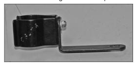
11. Install the oil fill tube retaining clip onto the "L" bracket (07093) with the hardware provided as shown.
