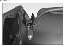
12. Using the spacer and hardware provided, install the oil filler tube retaining assembly onto the heat shield as shown.
