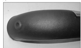
30. Remove the K&N® intake tube from the vehicle and drill a 3/4" hole at the marked location. Install the supplied grommet into the drilled hole. Be sure there are no shavings in the intake tube and then reinstall the K&N® intake tube into the vehicle and secure with the provided hose clamps.
