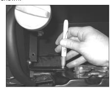
16b. Using a marker, mark the bolt hole location on the hood latch support bracket as shown.
