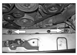
6. Remove the two air box mounting grommets shown.
