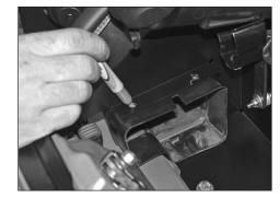
19. Mark the location of the holes in the heat shield on the fresh air supply duct as shown.
