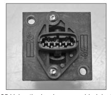
25. Using the hardware provided, install the mass air sensor onto the adapter plate as shown.
