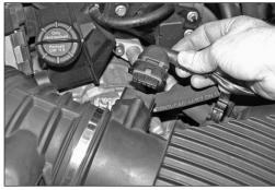
2. Depress the locking tab and disconnect the mass air sensor electrical connection. Unclip the mass air sensor wiring harness from the air box.
