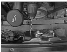
16c. Drill a 1/4"id hole into the hood latch support at the location marked in step 16b.
