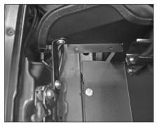
16f. Secure the heat shield to the "L" bracket (010040) installed in step 16e with the provided hardware.
