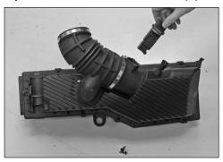
23. Using the T20 Torx wrench provided, remove the two screws, which secure the mass air sensor to the stock intake assembly. Remove the mass air sensor from the stock intake as shown.
