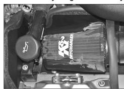
35. Install the K&N® filter onto the intake tube and secure with the provided hose clamp. Snap the stock oil fill tube into the retaining clip.
