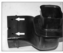
20. Drill two 3/8"id holes at the marked location on the fresh air supply duct.
