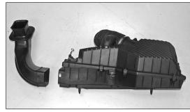
17. Remove the fresh air supply duct from the factory air box as shown.
