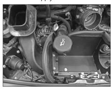
21. Using the hardware provided, bolt the fresh air supply duct to the heat shield as shown.
