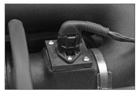
33. Connect the mass air sensor electrical connection as shown.
