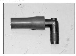
28. On vehicles with "TIPTRONIC" equipped vehicles, install the supplied silicone hose onto the 90° hose mender as shown.
