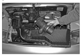
5. Remove the complete air box assembly from the vehicle as shown.
