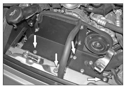
16. Install the heat shield assembly into the vehicle so that the inserted nuts go into the 3/4" air box mounting holes in the body. Tighten the mounting bolts and install the supplied mounting bolt through the "L" bracket into the body and tighten.
