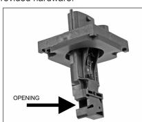
26a. Be sure to install the mass air sensor with the opening towards the filter end of the tube.
