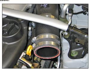
19. Install the silicone hose (08690) onto the end of the K&N $^{\odot}$  intake tube with the provided hose clamps.
