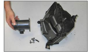
8. Remove the four bolts, which secure the mass air sensor to the factory air box and then separate the mass air sensor from the air box.
