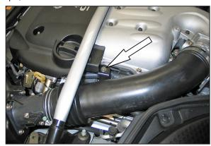
3. Remove the bolt, which secures the stock intake tube to intake manifold.
