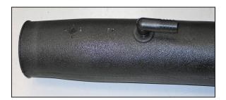
16. Install the provided 90 deg. fitting into the grommet that was installed onto the K&N<sup>®</sup> intake tube in step #15.
