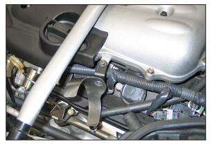
14. Install the saddle bracket assembly onto the engine using the bolt removed in step #3 as shown.
