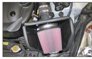
21. Install the Air Filter / mass air sensor assembly onto the K&N® intake tube, slide the silicone hose onto the mass air sensor housing and secure with the provided hose clamp as shown.
