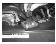
31. Reconnect the mass air sensor electrical connection.
