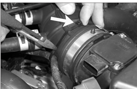
3. Lift up on the release tab to remove the factory zip-tie, as this will be reused in a later step.
