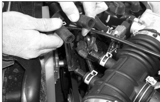
5. Remove the two hoses from the intake tube.
