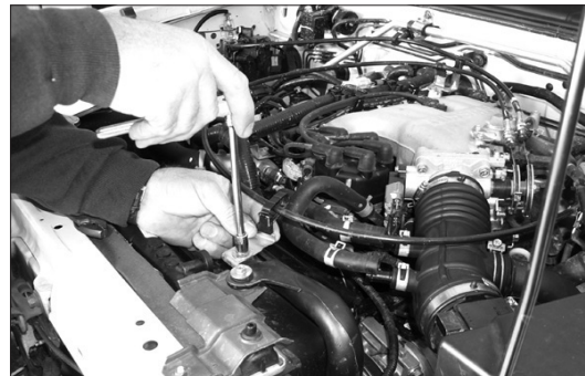
6. Disconnect the throttle cable bracket using a 10mm socket.
