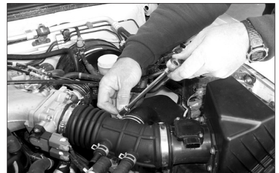
7. Loosen clamp on the resonator tube using a 10mm socket.
