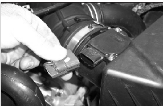
2. Disconnect the mass air sensor electrical connection.
