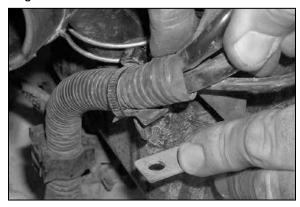
18. Using pliers, remove the wire loom clip.
