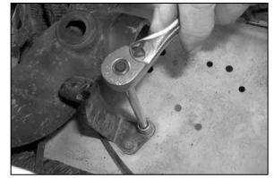
14. Remove the front support bracket using a 10mm socket.
