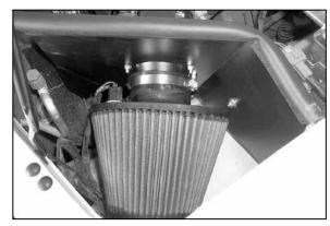
39. Install RX-4750 air filter element and secure with hose clamp using an 8mm socket or nut driver. NOTE: Drycharger® air filter wrap; part # RF-1042DK is available to purchase separately.
