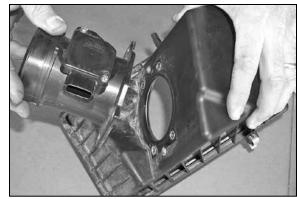
21. Remove the four bolts from mass air sensor housing using a 10mm socket and detach from airbox.
