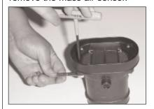
9. Attach the adapter to the mass air sensor and secure it using the hardware provided.
