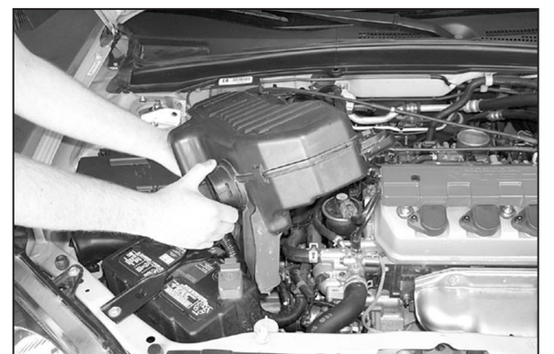
9. Detach the air inlet rubber boot and remove the resonator box.
