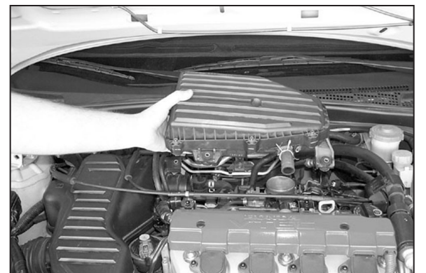
7. Pull upward firmly on the airbox to release it from the throttle body and remove.
