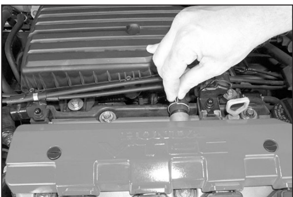
3. Detach the crankcase vent hose from the vent fitting on the valve cover.
