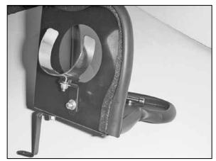
12. Attach the saddle bracket assembly to the heat shield using the hardware provided. **NOTE: Do not tighten completely at this time.**
