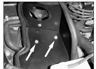
16. Attach the heat shield to the rubber mounted studs on the "Z" bracket using the hardware provided.
