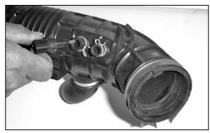
2. Disconnect the air temperature sensor electrical connection.
