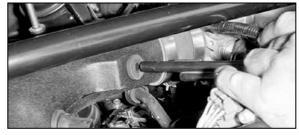
21. Insert the crankcase vent hardline into the grommet in the K&N $^{\mbox{\tiny $\$$}}$  intake tube.
