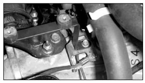
15. Attach the "Z" bracket to the transmission hanger using the bolt removed in the previous step.
