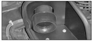
22. Install the adapter onto the K&N® intake tube.
