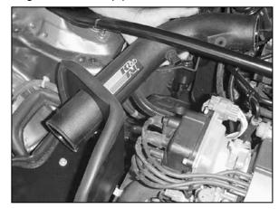
18. Install the K&N<sup>®</sup> intake tube, feeding the straight end through the hole in the heat shield.
