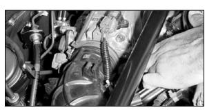
4. Loosen the hose clamp on the intake tube at the throttle body.
