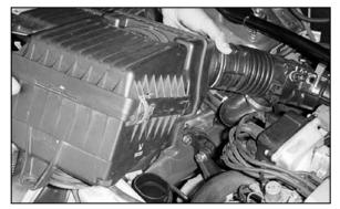
6. Detach the intake tube from the throttle body, pull upward firmly on the airbox to release it from it's retaining grommet and remove the entire air intake assembly.
