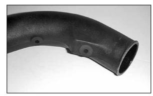
7. Insert the two grommets provided into the holes in the  $K\&N^{\circledast}$  intake tube.
