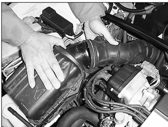
3. Detach the intake tube from the airbox.
