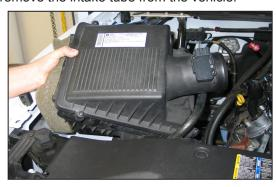
7. Pull up and remove the air box assembly from the vehicle as shown.
