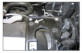
10. Remove the air box mounting grommet show.
