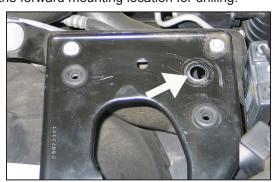
13. Remove the heat shield assembly and drill a 5/8"hole at the marked location.
