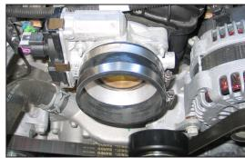
18. Install the provided silicone hose (#08761) onto the throttle body and secure with the provided hose clamp.
