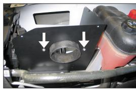
16. Install the filter adapter into the heat shield and secure with the provided hardware.
