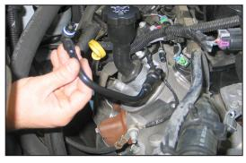
8. Rotate the crank case vent line on the valve cover, and then release the locking tab and remove the crank case vent line from valve cover port.
