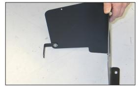
9. Install the heat shield mounting bracket (#010031) onto the heat shield as shown using the provided hardware.
