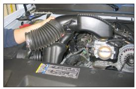
6. Loosen the two hose clamps which secure the intake tube to the throttle body and air box, then remove the intake tube from the vehicle.
