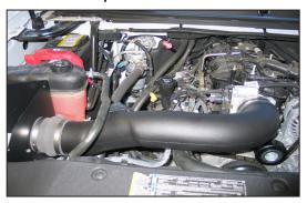
24. Install the K&N® intake tube into the silicone hose at the filter adapter and then into the silicone hose at the throttle body and secure with the provided hose clamps.
