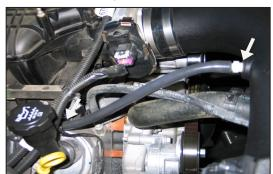
25. Install the provided silicone crank case vent hose onto the valve cover vent port and then to the  $\frac{1}{1}$  npt fitting in the K&N® intake tube as shown.
