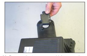
20. Remove the two screws which secure the mass air sensor to the factory air box and then remove the sensor from the air box.
