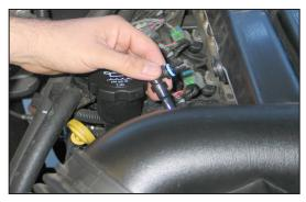
5. Disconnect the crank case vent line from the intake tube plenum as shown.
