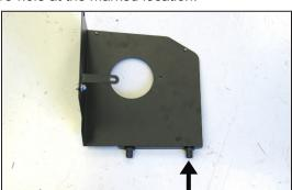
14. Install the remaining 5/16" inserted nut into the heat shield and secure with the provided hardware.
