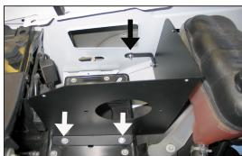
15. Reinstall the heat shield assembly, secure the mounting bracket to the inner fender with the provided hardware and then secure the two inserted nuts to the air box mounting tray.
