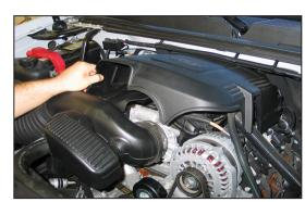
3. Lift up and remove the engine cover from the engine as shown.
