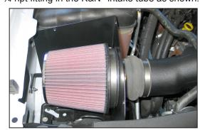
26. Install the K&N® air filter onto the filter adapter and secure with the provided hose clamp.
