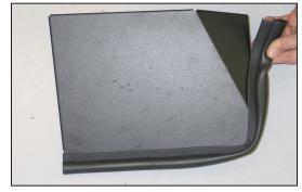
27. Install the provided edge trim onto the air filter cover as shown.
