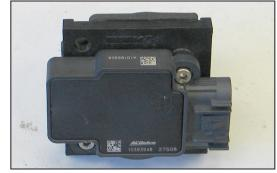
21. Install the mass air sensor into the K&N® mass air sensor adapter and secure with the provided hardware.
