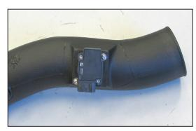
22. Install the mass air sensor assembly into the K&N® intake tube and secure with the provided hardware.
