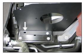
12. Set the heat shield assembly into position on the air box mounting tray so that the inserted nut sets into the air box mounting grommet hole. Mark the forward mounting location for drilling.
