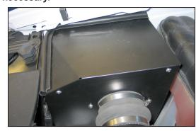
28. Install the air filter lid onto the heat shield and secure with the provided hardware.
