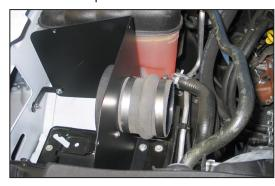
17. Install the silicone hose (#08418) onto the filter adapter and secure with the provided hose clamp.
