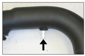
23. Install the provided  $\frac{1}{4}$ "NPT fitting into the K&N® intake tube as shown.
