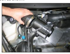
5. Loosen the hose clamp and then disconnect the stock intake tube from the air box.
