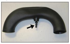
11. Install the provided crank case quick connect fitting into the K&N® intake tube as shown.
