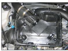
15. Install the air box onto the engine, connect the intake tube and secure with the provided hose clamp. Reinstall the retaining clips to secure the front of the air box. Reconnect the fresh air inlet tube to the air box.
