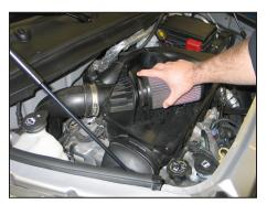
3. Remove the stock air filter from the air box as shown.
