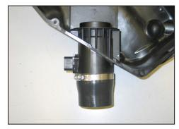
14. Install the provided silicone hose (08429) onto the factory air box and secure with the provided hose clamp.
