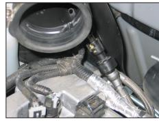
8. Release the crank case vent tube from the fitting on the stock intake tube.
