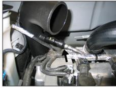
13. Connect the crank case vent hose to the quick connect fitting.
