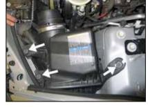
9. Remove the three bolts which retain the air box.
