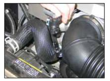
4. Release the crank case vent clip and then disconnect the crank case vent hose from the intake tube a shown.
