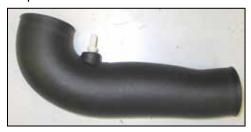
20. Install the crank case vent fitting into the K&N<sup>®</sup> intake tube as shown.
