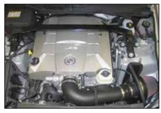
25. Reinstall the engine cover and radiator cover. Secure the radiator cover with the factory retainers.
