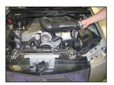
5. Loosen the hose clamps which secure the intake tube to the throttle body and air filter, then remove the intake tube from the vehicle as shown.
