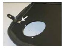
15. Install the heat shield mounting bracket (010127) onto the heat shield as shown using the provided hardware.
