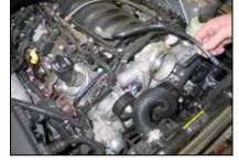
7. Remove the factory crank case vent hose from the valve cover.
