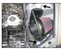
18. Install the heat shield assembly into the engine compartment and secure with the provided hardware.
