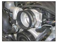
19. Install the silicone hose (08625) onto the throttle body and secure with the provided hose clamp.
