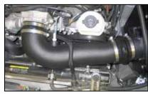
22. Install the K&N<sup>®</sup> intake tube onto the mass air sensor and then into the silicone hose on the throttle body. Secure the intake tube with the provided hose clamps.
