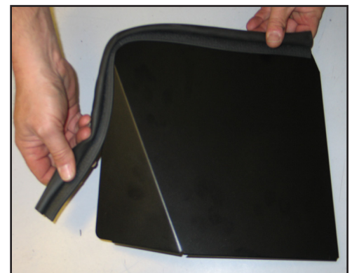
23. Install the 20" piece of edge trim onto the filter cover as shown. NOTE: Some trimming of the edge trim may be necessary.
