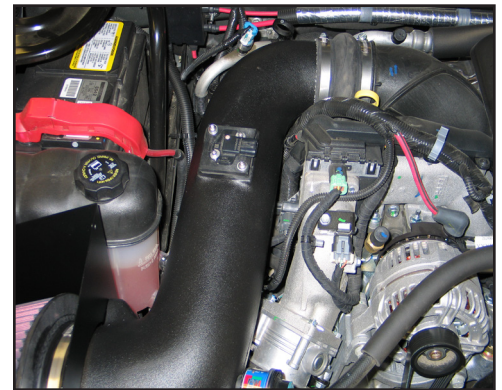
21. Install the K&N® Intake Tube into the silicone hose at the turbo inlet and into the heat shield, then secure the K&N® Intake Tube with the provided hose clamp and hardware as shown.
