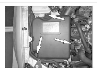
4. Loosen the three screws which secure the upper air box.
