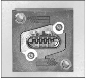
15. Install the mass air sensor into the mass air adapter and secure with the provided hardware.
