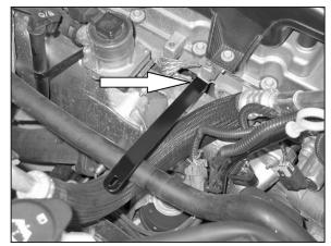
12. Install the tube mounting bracket (26632) onto the engine at the ground cable location and secure with the bolt removed in step #11.
