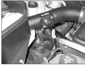
19. Cut the air injection hose at the location marked in step #18. Then install the hose onto the K&N® intake tube and secure with the provided hose clamp
