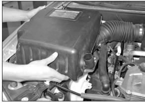
5. Remove the upper air box cover as shown.
