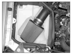
20. Install the K&N® air filter onto the K&N® intake tube and secure with the provided hose clamp. NOTE: Drycharger® air filter wrap; part # RX-4730DK is available to purchase separately.
