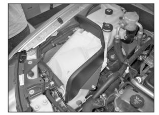
10. Install the heat shield onto the coolant reservoir with the hardware provided.
