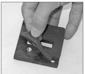
14. Install the adapter gasket onto the adapter plate as shown.
