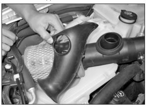
6. Remove the fresh air supply duct.
