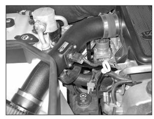
21. Reconnect the mass air sensor electrical connection as shown.
