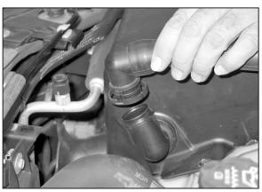
3. Depress the locking tabs and disconnect the air injection hose.
