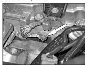
11. Remove the engine ground strap bolt shown. **NOTE: This bolt will be reused.**
