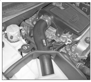
17. Install the K&N® intake tube assembly into the silicone hose at the throttle body and align it with the mounting bracket installed in step #12. Then secure the tube with the provided hose clamp and hardware.
