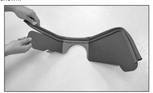
9. Install the provided edge trim onto the heat shield as shown.
