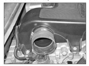
13. Install the provided silicone hose (08051) to the throttle body and secure it with the provided hose clamp.
