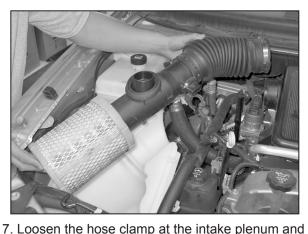
then remove the complete intake system.
