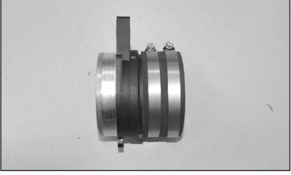
26. Install the silicone hose (08615) onto the mass air sensor as shown and secure with the provided hose clamp.
