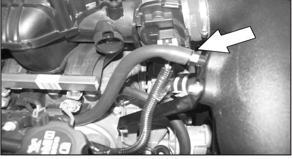
25. Connect the supplied crankcase vent hose onto the valve cover and then connect to the intake tube as shown.
