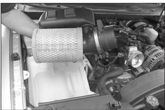
10. Remove the filter and mass air sensor assembly from the vehicle as shown. NOTE: K&N Engineering, Inc., recommends that you do not discard your factory air intake.
