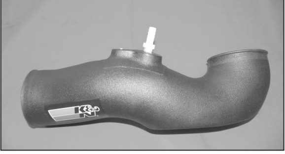
23. Install the provided vent fitting into the intake tube as shown. NOTE: Plastic NPT fittings are easy to cross thread. Install the vent fitting "hand" tight, then turn it two complete turns with a wrench.
