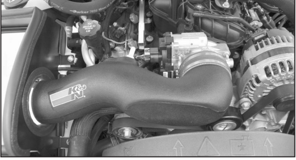
24. Install the intake tube into the silicone hose at the throttle body and align with the mounting bracket installed in step #20. Secure the tube with the provided hose clamp and hardware. Do not completely tighten at this time.
