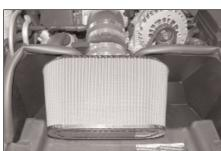
23. Install the air filter onto the mass air sensor and secure with the provided hose clamp.
