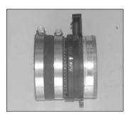
16. Install the provided silicone hose (08615) onto the engine side of the mass air sensor and secure with the provided hose clamp.
