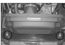
7. Remove the two bolts, which secure the air box to the core support.
