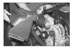
8. Loosen the hose clamp that secures the stock intake tube to the throttle body, and then remove the complete intake assembly from the vehicle.
