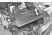
6. Lift the core support cover up and remove it from the vehicle.
