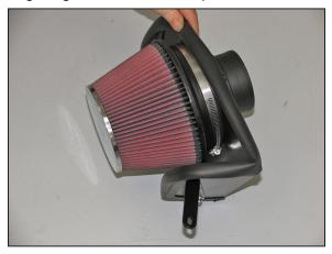
14. Install the K&N® air filter onto the heat shield assembly and secure with the provided hose clamp as shown.
