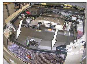
20. Reinstall the radiator cover onto the radiator core support and reinstall the clips removed in step #2
