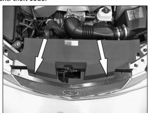
2. Release the two locking pins shown which secure the radiator cover to the radiator core support.
