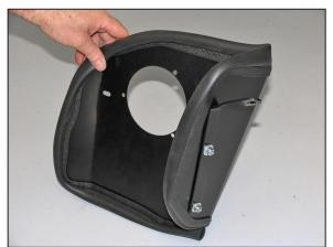
10. Install the heat shield mounting bracket onto the heat shield as shown with the provided hardware
