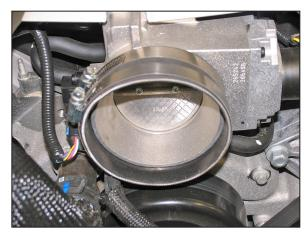
17. Install the silicone hose (08755) onto the throttle body and secure with the provided hose clamps.
