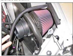
16. Install the provided button head allen and fender washer onto the core support to retain the inner splash shield as shown.
