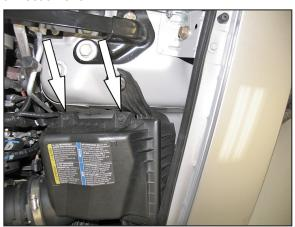
6. Loosen the two screws, which secure the air box lid to the air box base.
