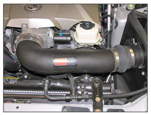
19. Install the K&N® intake tube onto the throttle body and mass air sensor as shown and secure with the provided hose clamp.
