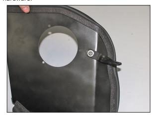
11. Install the heat shield mounting bracket onto the heat shield as shown with the provided hardware.
