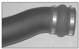
17. Install the silicone hump hose (08176) onto the intake tube as shown and secure with the provided hose clamps as shown.
