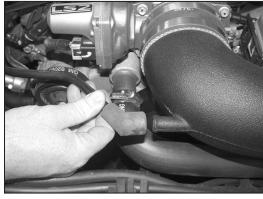
19. Install the crank case vent hose onto the  $K\&N^{\otimes}$  intake tube as shown.
