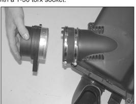
9. Loosen the hose clamp that secures the mass air sensor to the factory air box, then remove the mass air sensor from the factory air box.
