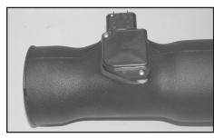
17. Install the mass air sensor assembly into the K&N® intake tube using the provided spacers and button head allen bolts provided.
