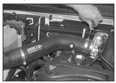
22. Install the K&N® intake tube into the silicone hose at the throttle body and through the heat shield so it rests onto the tube-mounting bracket assembly, then secure with the provided hose clamps.
