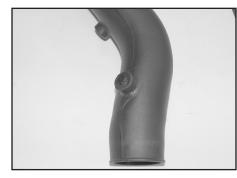
18a. On vehicles not equipped with a fuel pressure regulator vent hose, install the provided NPT plug into the K&N® intake tube as shown.
