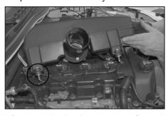
8. Remove the intake resonator from the engine as shown.
