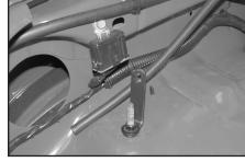
13. Install the "L" bracket (070602) onto the stock airbox mounting stud using the factory airbox retaining nut.
