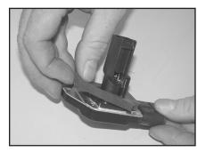
16. Apply provided gasket to mass air sensor as shown.
