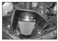
27. Install the air filter assembly onto the K&N<sup>®</sup> intake tube and secure with the provided hose clamp.
