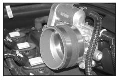
9. Install the silicone hose (08690) onto the throttle body and secure with the provided hose clamp as shown.
