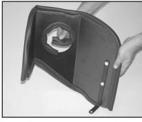
12. Install the edge trim onto the inner hole on the heat shield as shown. Trim if needed.
