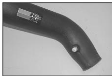
18. Install the provided  $\frac{1}{4}$ " NPT vacuum fitting into the K&N® intake tube as shown.
