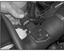
28. Reconnect the mass air sensor electrical connection.
