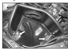
14. Install the heat shield into the vehicle using the hardware provided and the factory airbox retaining nut.
