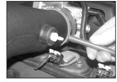
23. On vehciles equipped with a fuel pressure regulator install the provided 4mm vacuum hose onto the fuel pressure regulator, then onto the ½" npt vacuum fitting on the K&N® intake tube.
