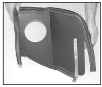
11. Install the edge trim onto the heat shield as shown.
