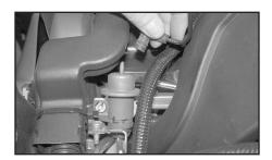
6. On vehicles equipped with a fuel pressure regulator disconnect the fuel pressure regulator vacuum hose from the fuel pressure regulator as shown.
