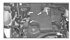
7. Loosen the two bolts that retain the intake resonator to the engine, and then loosen the hose clamp at the throttle body.
