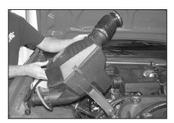
5. Lift up the airbox and remove it from the vehicle. NOTE: K&N Engineering, Inc., recommends that customers do not discard factory air intake.
