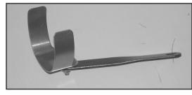
20. Install the saddle clamp onto the tubemounting bracket with the provided hardware as shown.
