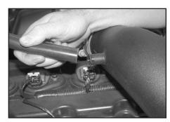
24. Install the provided crankcase vent hose onto the valve cover, then onto the  $K\&N^{\circledR}$  intake tube as shown.
