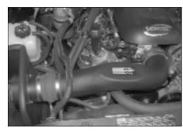
12. Install the K&N intake tube onto the mass air sensor, then secure the other end onto the throttle body as shown.
