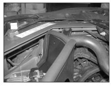
24. Remove the radiator mounting bolt shown.
