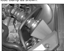
36. Install the air filter assembly onto the mass air sensor and secure with the provided hose clamp as shown.
