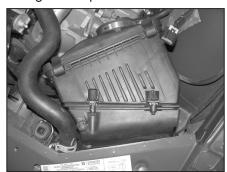
8. Loosen the two air filter housing mounting bolts shown.
