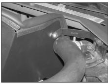
25. Install the K&N® bracket (010056) onto the heat shield and radiator mount as shown.
