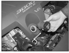
2. Twist the oil fill pipe counter clockwise and remove it from the valve cover.
