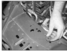
21. Install the provided inserted nuts into the airbox mounting grommet holes exposed in step #20.
