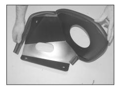
16. Install the provided edge trim onto the heat shield as shown.
