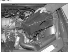
9. Tilt the air filter housing in, then lift to remove the filter housing from the mounting tabs.
