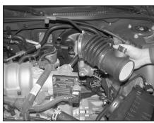
6. Loosen the hose clamps, which secure the stock intake tube to the throttle body and the mass air sensor to the stock airbox. Remove the intake tube assembly from the vehicle as shown.
