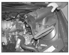
12. Pull firmly up on the engine processor housing to release it from the mounting tabs, then remove the housing from the vehicle.
