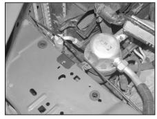
20. Remove the two airbox mounting grommets shown by pulling them up out of the holes in the fender apron.
