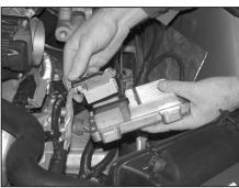
11. Unlock the engine processor electrical connections and then disconnect the connections from the processor.
