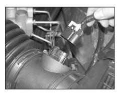
4. Depress the locking tab on the mass air sensor electrical connection, and then pull up to separate the mass air sensor electrical connection.
