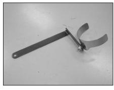
17. Install the saddle clamp onto the tube mounting bracket (010093) with the provided hardware as shown.
