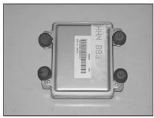
14. Install the rubber mounted studs to the processor with the provided hardware as shown.
