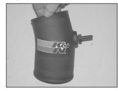
27. Install the provided NPT into the  $K\&N^{\scriptsize @}$  intake tube as shown.
