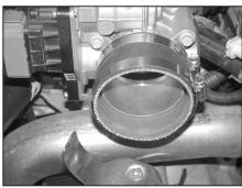
26. Install the silicone hose (08690) onto the throttle body and secure with the provided hose clamps as shown.
