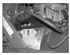
22. Set the heat shield and engine processor assembly into position on the fender apron. Using the bolts provided, fasten the processor assembly the heat shield to the inserted nuts in the fender apron as shown.
