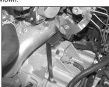
19. Install the saddle clamp assembly onto the stud exposed in step #18 and secure with the provided hardware.
