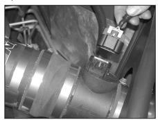
39. Reconnect the mass air sensor electrical connection.
