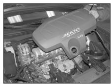
3. Lift the engine cover to remove it from the engine.
