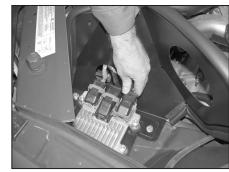
23. Pass the engine wiring harness through the hole in the heat shield, then reconnect the harness to the engine processor.
