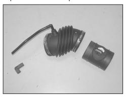
29. Loosen the hose clamp, which secures the mass air sensor to the stock intake tube, and then remove the mass air sensor and vent hose elbow from the stock intake tube.
