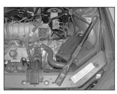
7. Remove the three body support brace mounting bolts shown, then remove the support brace from the engine compartment.
