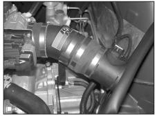
31. Install the mass air assembly onto the  $K\&N^{\otimes}$  intake tube and secure with the provided hose clamp as shown.
