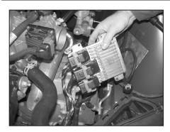
10. Unlock the engine processor from its mounting tabs and lift it out from the processor housing.
