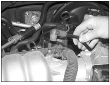
5. Disconnect the vent tube from the intake manifold.
