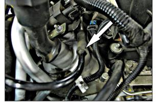
9a. On vehicles equipped with a crank case vent hose, remove the factory vent hose from the valve cover vent port shown.
