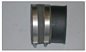
21. Install the supplied silicone hose (08625) onto the small diameter end of the "EH" K&N $^{\circ}$  intake tube.
