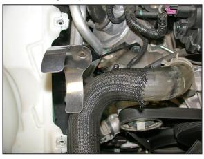
13. Install the tube bracket assembly onto the engine using the hardware provided. NOTE: The supplied bolt threads into the threaded hole in the engine vacated by the wire harness clip in step #11.
