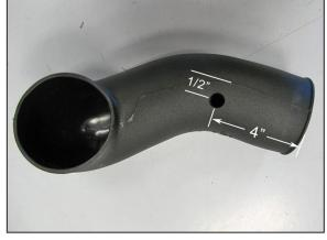
18a. On vehicles equipped with a crank case vent, mark the tube 4" back from the end of the tube and  $\frac{1}{2}$ " below the mold seam then drill a 5/8"id hole.
