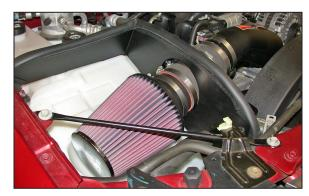
24. Re-install the core support brace removed in step #4 with the stock hardware. **NOTE: Adjust the air filter and intake tube at this time for minimum of 1/2" clearance then tighten the hose clamps.**
