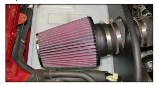
23. Install the K&N<sup>®</sup> air filter onto K&N<sup>®</sup> intake tube and secure with the provided hose clamp.
