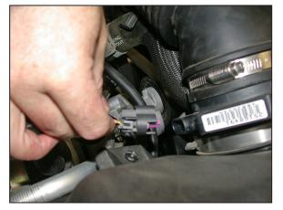
2. Depress the locking tab on the mass air sensor electrical connection and then separate the connector from the mass air sensor.
