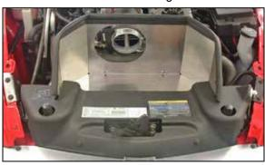
17. Reinstall the core support cover removed in step #5 and secure with the retaining clips removed step #3 and the factory nuts removed in step #4.
