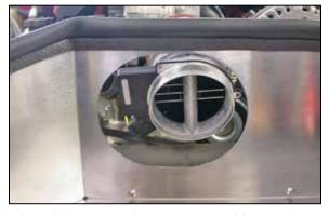
15.Install the mass air sensor assembly onto the  $K\&N^{\tiny \circledcirc}$  intake tube and secure with the provided hose clamp.
