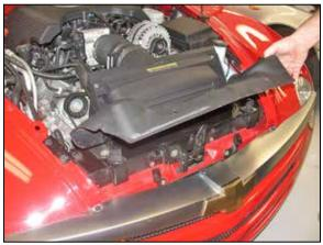
5. Lift the core support cover up and remove it from the vehicle.
