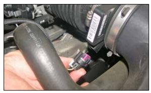
2. Disconnect the mass air sensor electrical connection.
