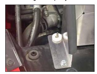
16. Install the two provided nylon spacers onto each side of the air box mounting studs as shown.
