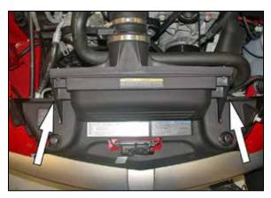
4. Remove the two 10mm nuts, which hold the core support cover onto the air box.
