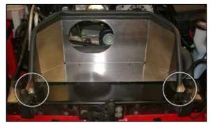
11. Install the heat shield assembly onto the air box mounting points and secure with the provided hardware.
