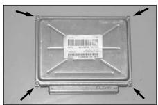
15. Remove the four processor cover plate bolts shown with a #27 Tork socket.
