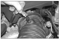
2. Unclip and disconnect the air temperature electrical connection.
