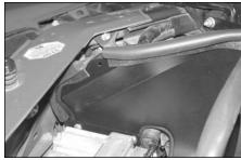
26. Remove the radiator mounting bolt and bracket shown.
