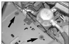
18. Remove the two air box mounting grommets shown by pulling them up out of the holes in the fender apron.
