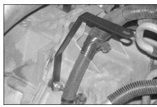
22. Install the K&N tube mounting bracket (07199) onto the stud exposed in step #21 and secure with the hardware provided
