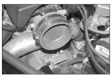
29. Install the silicone hose (08621) onto the throttle body and secure with the provided hardware as shown.
