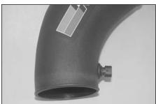
32. Install the air temperature sensor into the K&N intake tube as shown.
