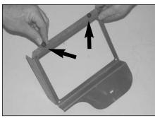
11. Install the rubber bumpers provided into the processor mounting bracket (010058) as shown.
