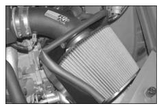
35. Install the K&N filter charger onto the intake tube and secure with the provided hose clamp.
