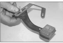
27. Place the K&N bracket (010056) behind the factory radiator bracket as shown.
