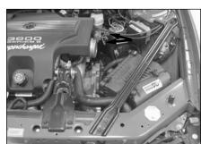
5. Remove the three body support brace mounting bolts shown, then remove the support brace from the engine compart-
