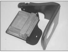
16. Install the engine processor onto the K&N heat shield and mounting bracket as shown.
