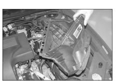
10. Pull firmly up on the engine processor housing to release it from the mounting tabs, then remove the hosing from the vehicle.
