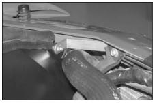
28. Reinstall the factory radiator bracket onto its original location with the K&N bracket (010056) so that the K&N bracket meets with the heat shield assembly and secure with the provided hardware.
