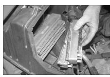
8. Loosen the center retaining bolts on the engine processor electrical connection and unplug the connectors from the engine processor.
