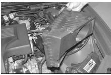
7. Tilt the air filter housing in, then lift to remove the filter housing from the mounting tabs.
