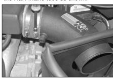
33. Install the K&N intake tube onto the throttle body, securing with the hose clamp provided, then secure the tube to the mounting bracket installed in step #22 with the provided 8mm bolt.
