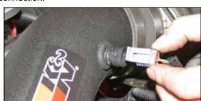
31. Reconnect the temperature sensor electrical connection.
