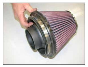
19. Install the radiused filter adapter into the K&N $^{\circ}$  air filter as shown. Secure with the provided hose clamp.
