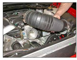
5. Loosen the two intake tube hose clamps, then remove the intake tube from the vehicle.
