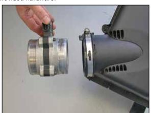
26. Loosen the hose clamp that secures the mass air sensor to the factory air box, then remove the mass air sensor from the factory air box.
