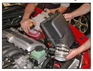
8. Have an assistant hold the coolant reservoir up, lift up on the air box assembly to release it from the retaining studs. Then remove the air box from the vehicle.
