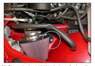
23. Secure the heatshield to the inner fender with the 6mm bolt provided.
