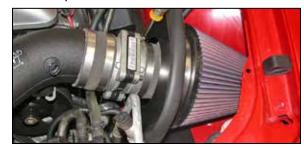
29. Install the air filter assembly onto the K&N<sup>®</sup> intake tube and secure with the provided hose clamp.
