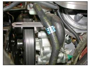
12. Install the tube bracket #010061 using the provided hardware.
