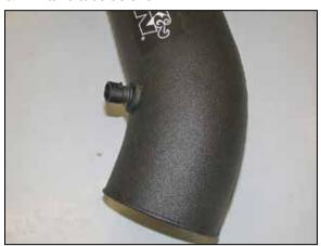
16. Install the air temperature sensor from step #14 into the grommet in the K&N® intake tube as shown
