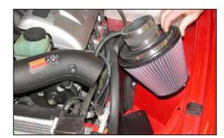
22. Set the heatshield assembly onto the inner fender, then set the air filter assembly between the heatshield and fender as shown.
