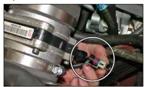
30. Reconnect the mass air sensor electrical connection.
