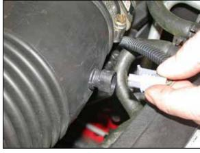
4. Release the air temp. electrical connection clip, then disconnect the electrical connection.
