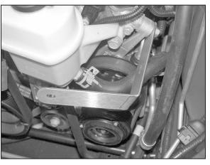
12. Install the K&N<sup>®</sup> "L" bracket (#07188) as shown with the bolt removed in step #11.
