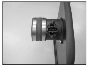
18. Install the silicone hose (#08690) onto the mass air assembly with the provided hose clamps as shown
