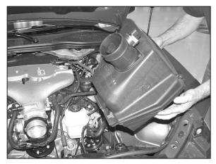
7. Remove the air box from the vehicle as shown. NOTE: K&N Engineering, Inc., recommends that customers do not discard factory air intake.
