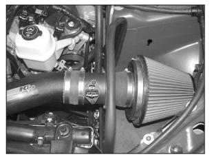
22. Install the filtercharger assembly onto the mass air sensor and secure with the provided hose clamp.
