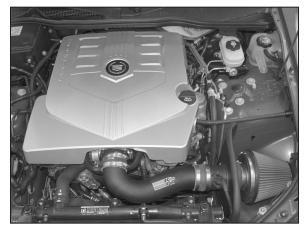
24. Reinstall the engine cover and oil cap removed in step #3.
