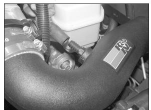
15. Install the crankcase vent hose onto the K&N®
