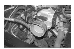
10. Install the provided silicone hose (08621) onto the throttle body with the provided hose
