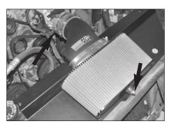
18. Align the intake tube for best clearance then tighten hose clamp at the throttle body and secure the filter to heat shield.
