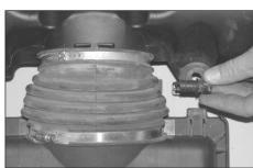
12. Remove the temp sensor from the factory air box as shown.
