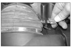
2. Disconnect the air temp sensor electrical connection.
