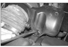
3. Pry up on the two tabs to release the clip that retains the resonator to the radiator
