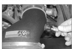
19. Reconnect the air temp sensor electrical connection.
