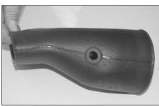
11. Install the grommet into the K&N intake tube as shown.
