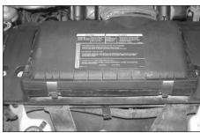
4. Release the two clips that retain the air box top to the air box base.
