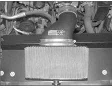
17. Install the K&N intake assembly onto the heat shield and throttle body.
