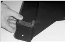
8. Install the rubber cushion onto the heat shield as shown.
