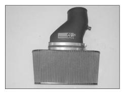
15. Install the K&N intake tube onto the filter charger as shown.
