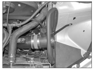
14. Install the heat shield assembly onto the vehicle, then attach intake tube to silicone hose and secure bracket to wheel well as shown.
