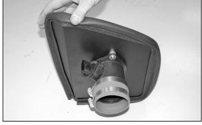
13. Install silicone hose (08434) onto the mass air assembly with the provided hose clamps as shown.
