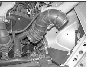
5. Loosen the lower hose clamp on the intake tube, then remove intake tube as shown.
