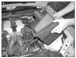
4. Remove air box from vehicle as shown.
