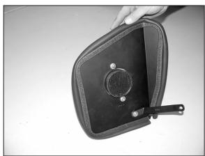
12. Attach the bracket onto heat shield with the provided hardware as shown.
