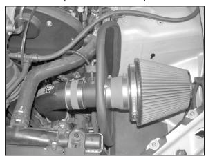
17. Install the K&N® filtercharger onto the mass air assembly as shown.
