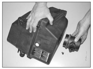
7. Remove the two screws that secure the mass air sensor to air box, then remove mass air sensor.
