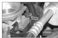
12. Using a 10mm socket remove the wire harness retaining clip nut at the front of the throttle body.
