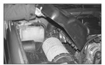
3. Release the over center clamps and remove the air box lid.
