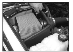
23. Install the air filter onto the mass air sensor and then tighten hose clamp.
