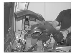
6. Detach the intake tube from the throttle body and mass air sensor then remove the intake assembly.
