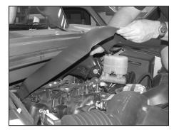
2. Remove the 8mm bolt that retains then engine cover onto the engine then remove the cover from vehicle.
