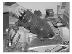
8. Remove the air box from vehicle as shown. NOTE: K&N Engineering, Inc., recommends that customers do not discard factory air intake. 11. Install the edge trim onto the heat shield. NOTE: Some trimming of the edge trim may be necessary.
