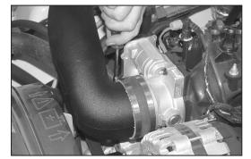
22. Align the intake tube with the throttle body then tighten the hose clamps.
