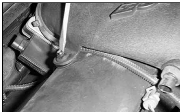
4. Release the push clips that retain the stock intake tube to the upper radiator cover.
