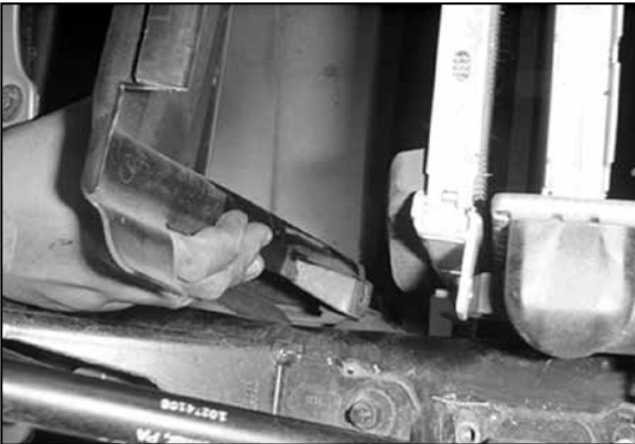
33. Pull firmly to release the radiator cover from its retaining clips.
