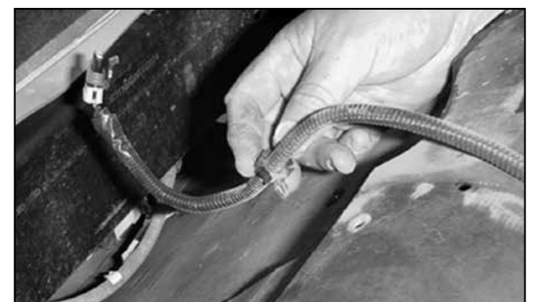
8. Detach the wiring harness retaining clip from the lower radiator cover.
