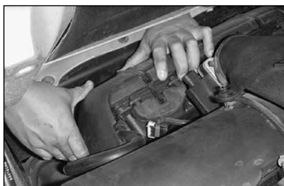
6. Pull the airbox towards the engine to release it from its mounting grommets.
