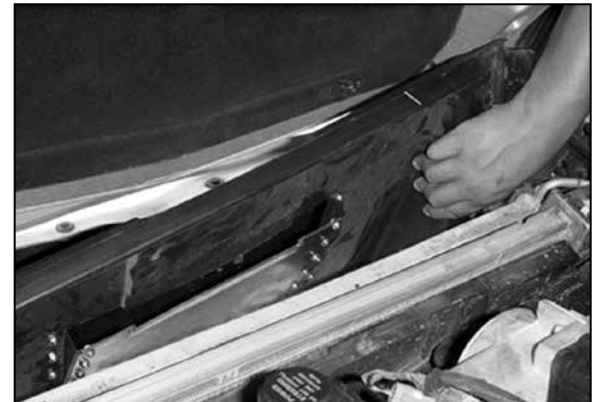
43. Reinstall the lower radiator cover.
