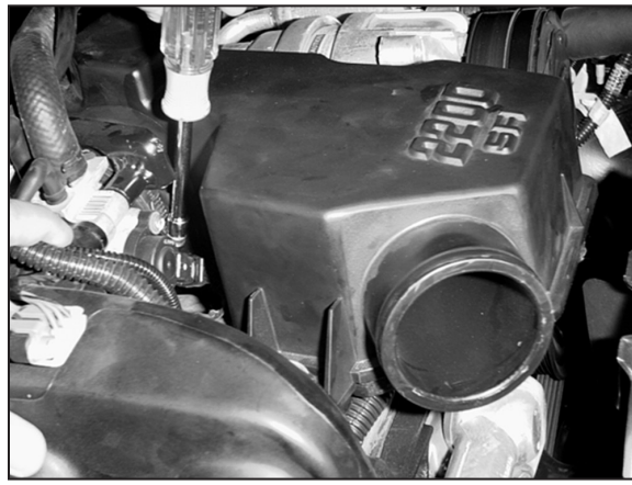
13. Loosen the hose clamp on the resonator at the throttle body.
