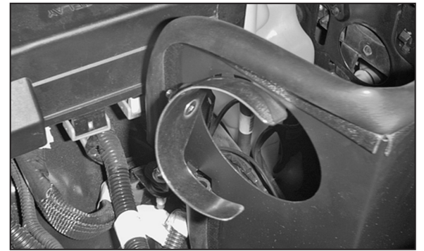
22. Install the saddle bracket assembly onto the airbox mounting stud and secure using the hardware provided. NOTE: Do not tighten completely at this time.
