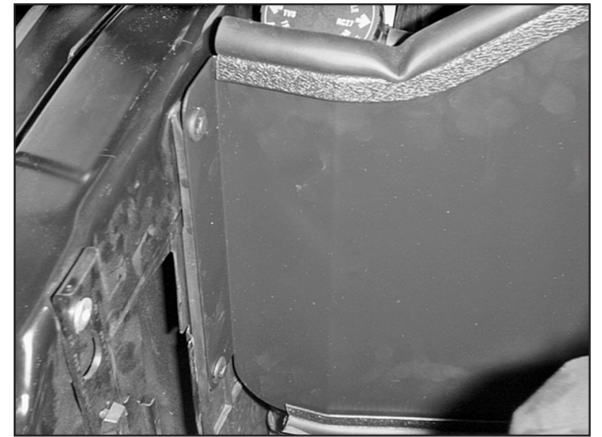
20. Secure the heat shield to the radiator core support using the clips removed in step 18.
