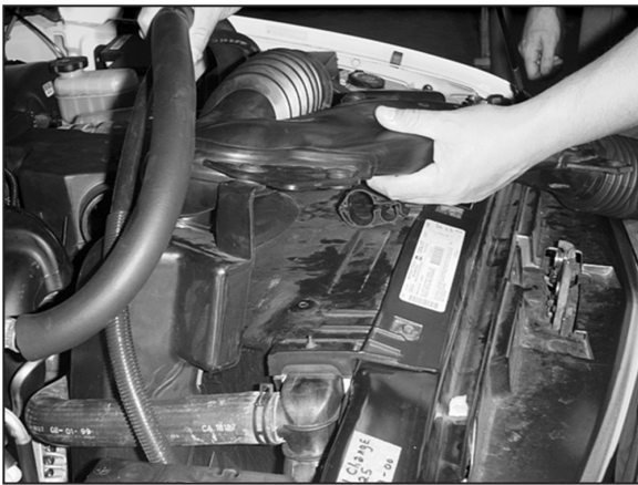
9. Remove the entire intake tube assembly.
