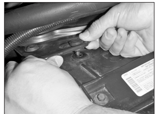
6. Pry up on the two push clips that retain the intake tube to the radiator shroud.
