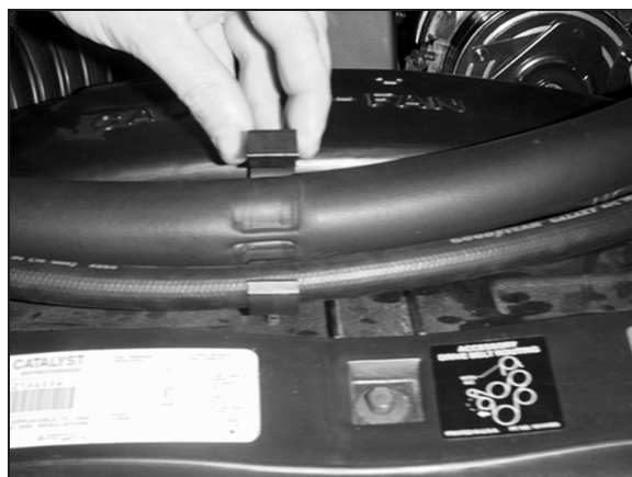
3. Detach the clip that retains the a/c lines to the radiator shroud.
