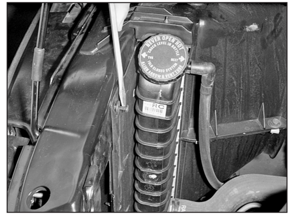
18. Pry up on and remove the two push clips from the radiator core support.
