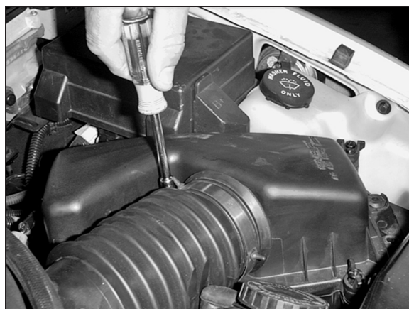
4. Loosen the hose clamp on the intake hose at the airbox.
