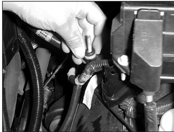
17. Install the 3/8" ID grommet onto the airbox mounting stud.
