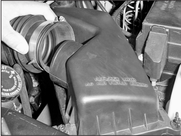
8. Detach the intake hose from the airbox.
