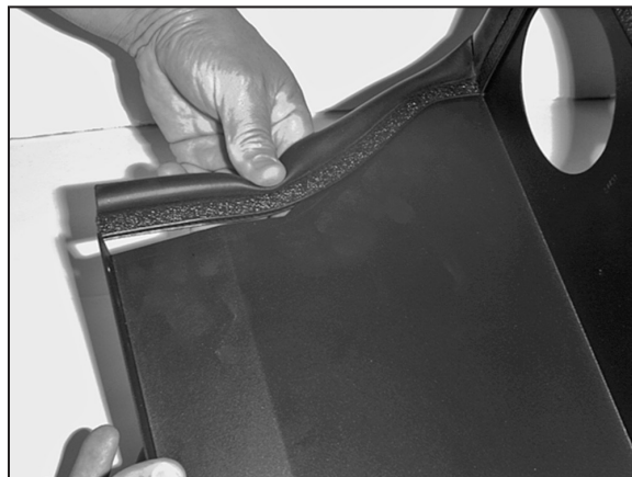
16. Install the trim seal onto the heat shield as shown.
