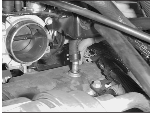
14. Detach the crankcase vent hose from the valve cover.
