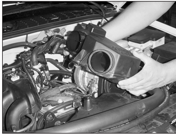
15. Detach the resonator from the throttle body and remove it.
