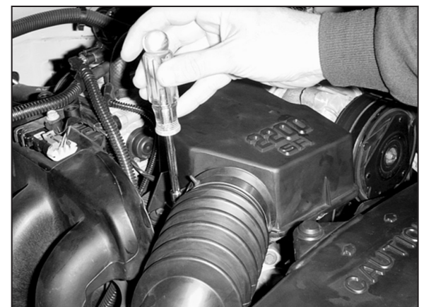
5. Loosen the hose clamp on the intake hose at the resonator.
