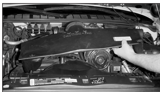
7. Pull firmly upward to release the air intake plenum from its grommets and remove complete assembly.
