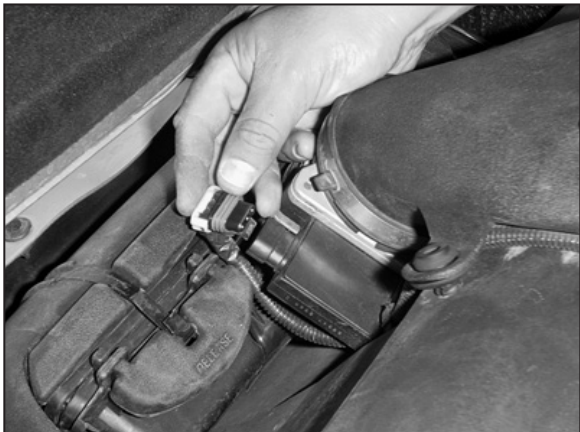
2. Disconnect the mass air sensor electrical connection.
