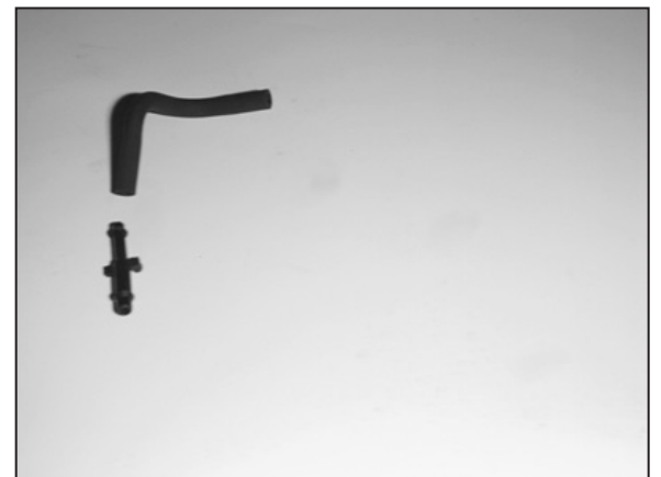
6. On models equipped with a fuel pressure regulator vacuum line, detach the vent from the vent hose.
