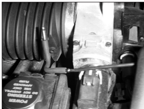
4. On models equipped with a fuel pressure regulator vacuum line, disconnect the vent from the intake hose.
