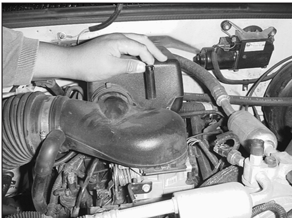
2. Loosen and remove the tall wing nut on the throttle body.
