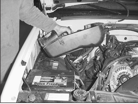
8. Remove the lower airbox assembly.
