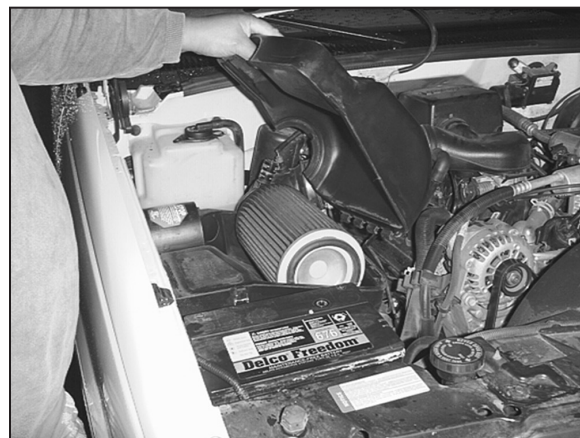
3. Release the over center clamps and remove the airbox lid.
