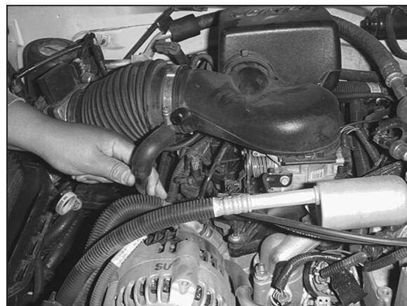
4. Disconnect the crankcase vent hose from the factory air intake tube.
