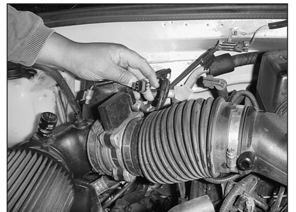
6. Disconnect the mass air sensor electrical connection.
