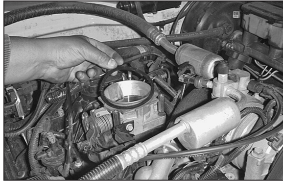
15. Install the neoprene gasket provided onto the throttle body flange.
