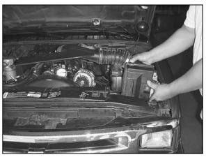
6. Remove the complete air intake assembly from the engine compartment.
