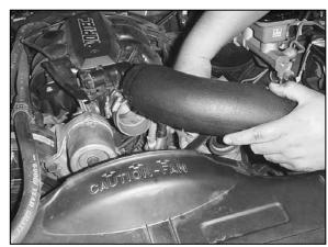
21. Install the K&N® intake tube, resting comfortably on the saddle/bracket and inserting the one end of the tube into the silicone hose. Reconnect the air temperature sensor electrical connection and insert the vent hose into the grommet hole located on the backside of the K&N tube.
