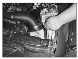
24. Install the air filter element onto the end of the intake tube. Position element for best clearance and tighten down using the provided hose clamp.
