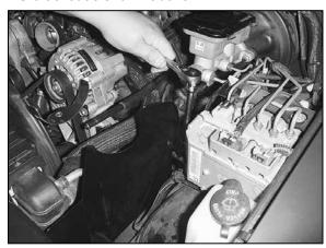
13. Install the heat shield as shown, with the factory ABS bracket bolt reinstalled.
