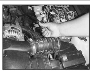
5. Remove the vent hose from the factory intake tube.
