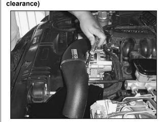
23. Install the hose clamp provided around intake tube and saddle and tighten as shown above.
