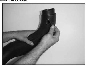
18. Install the two grommets provided into the  $K\&N^{\otimes}$  intake tube as shown above.
