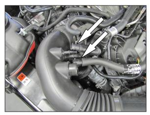
7. On vehicle equipped with an EVAP vent line, disconnect the EVAP vent line from the factory intake tube. Disconnect the crank case vent hose from the factory intake tube.
