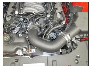
14. Install the K&N<sup>®</sup> intake tube into the hose at the air box and then into the hose at the throttle body. Adjust the tube for proper fitment and then secure with the provided hose clamps.
