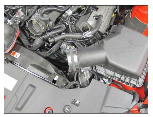
12. Install the provided coupling hose (08536) onto the air box outlet and secure with the provided hose clamp.
