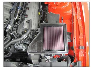
10 Remove the factory air filter and replace with
