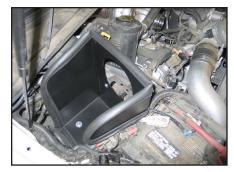
13. Install the heat shield assembly into position so that the rubber mounted studs protrude through bottom of the heat shield. Secure the heat shield with the provided hardware and the factory battery tray bolt removed in step #12.
