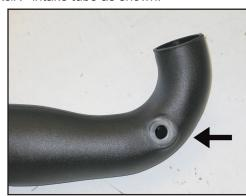
16. Install the supplied crank case grommet into the K&N® intake tube as shown.
