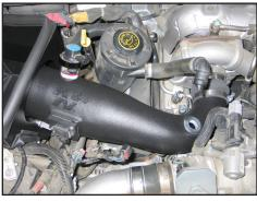
22. Install the K&N® intake tube assembly into the heat shield and slide the silicone hose onto the turbo inlet. Secure the intake tube to the mounting bracket on the heat shield with the provided hardware and then position the silicone hose onto the turbo and secure with the hose clamps.
