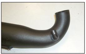
16a. On models that have the crank case vent fitting attached to the stock intake tube, install the supplied 90° vent fitting into the grommet as shown.
