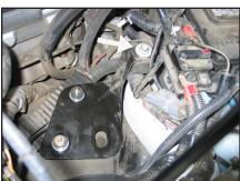
12. Remove the battery tray mounting bolt shown. **NOTE: This bolt will be reused.**
