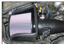
25. Install the K&N® Air Filter onto the K&N® intake tube and secure with the hose clamp.
