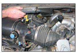
6. Unhook the warm air inlet tube from the fire wall as shown.
