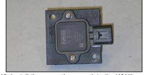
19. Install the mass air sensor into the K&N® mass air sensor adapter and secure with the provided hardware.
