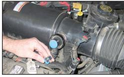
3. Disconnect the filter minder electrical connection.
