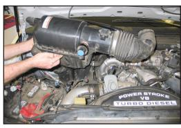
7. Lift up firmly on the complete air box assembly to dislodge it from the mounting grommets and then remove the complete air box and intake tube assembly from the vehicle.
