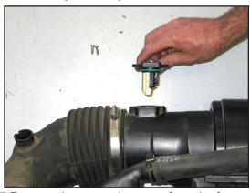
17.Remove the mass air sensor from the factory air filter housing.
