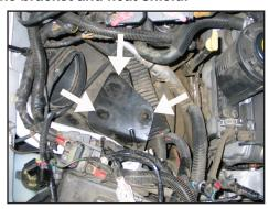
10. Remove the three air box mounting grommets shown from the mounting tray.
