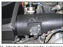
24. Attach the filter minder extension harness provided into the factory harness and then connect the open end to the filter minder.
