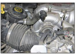
4. Clip the band clamp which secures the crank case breather hose to the intake tube. Then disconnect the breather hose and fitting from the intake tube as shown.
