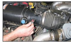
2. Disconnect the mass air sensor electrical connection and unclip the wiring harness from the air box as shown.
