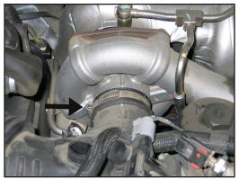
5. Loosen the hose clamp which secures the intake tube to the turbo inlet.
