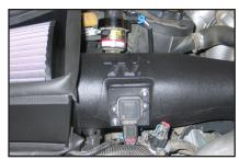
26. Reconnect the mass air sensor electrical connection.
