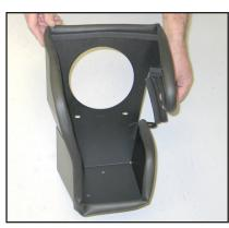
8. Install the provided edge trim onto the heat shield as shown.
