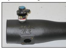
15. Install the filter minder and grommet into the K&N® intake tube as shown.
