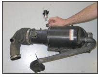
14. Remove the filter minder and grommet from the factory air filter housing as shown.
