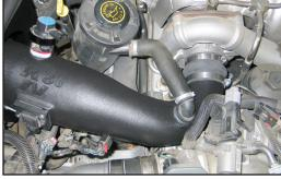
23. Insert the crank case vent fitting into the grommet in the K&N® intake tube.
