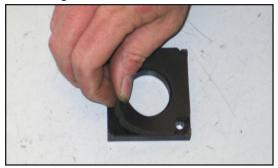
18. Install the provided gasket onto the K&N® mass air sensor adapter.
