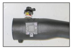
20. Install the mass air sensor assembly onto the K&N® intake tube as shown and secure with the provided hardware as shown.
