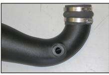
21. Install the provided silicone (087121) hose onto the  $K\&N^{\otimes}$  intake tube with the hose clamps provided as shown.
