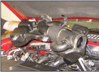
6. Remove the factory inlet tube as shown.
