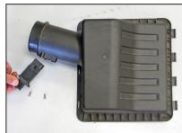
10. Remove the two screws securing the mass air sensor, then remove the mass air sensor from the upper air box housing as shown.
