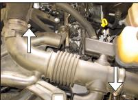
5. On the factory inlet tube, loosen the hose clamps at the upper air box housing and at the throttle body inlet.
