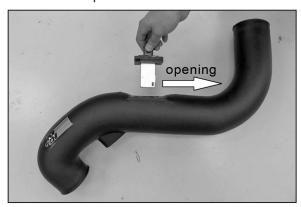
26. Install the mass air sensor assembly into the  $K\&N^{\circledcirc}$  intake tube and secure with the provided hardware.
