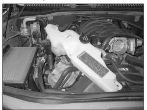
Lift and position the coolant recovery tank on the engine to gain access to the lower air box.
