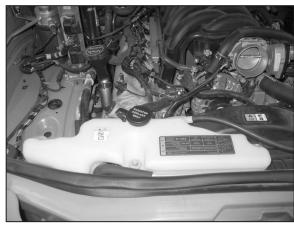
11. Reinstall the coolant recovery tank and secure with the factory bolts removed in step #8.
