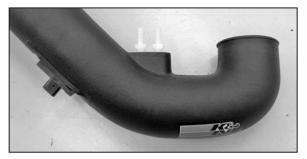
27. Install the two npt vent fittings into the K&N® intake tube as shown.
