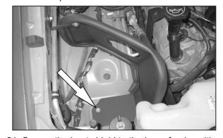
21. Secure the heat shield to the inner fender with the bolt removed in step #13 and the inserted nut and bolt.
