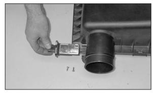
23. Remove the two screws that secure the mass air sensor to the stock air box and then remove the mass air sensor.
