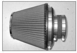
32. Install the silicone hose (08630) onto the air filter adapter and secure with the provided hose clamp.
