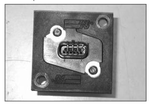
25. Install the mass air sensor into the adapter and secure with the provided hardware.
