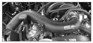
28. Install the K&N® intake tube into the silicone hose at the throttle body and align with the mounting bracket installed in step #16. Secure the intake tube with the hose clamp and supplied hardware.
