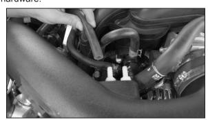
29. Install the supplied shorter crank case vent line onto the fitting on the valve cover and then onto the npt fitting installed in the K&N® intake tube.
