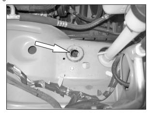
13. Remove the washer bottle mounting bolt shown.
