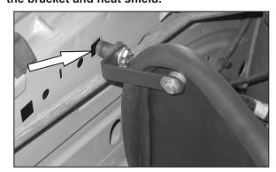
20. Install the heat shield assembly into the vehicle so that the inserted nut will fit into the hole in the inner fender panel.
