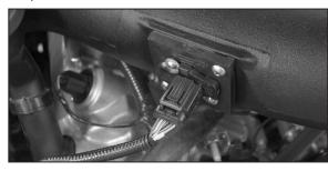
34. Reconnect the mass air sensor electrical connection.
