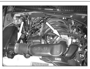
5. Loosen the hose clamps that secure stock intake tube to the throttle body and air box shown.
