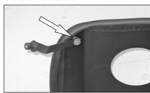
19. Attach the mounting bracket assembly to the heat shield with the provided hardware as shown. NOTE: Be sure to position the spacer between the bracket and heat shield.
