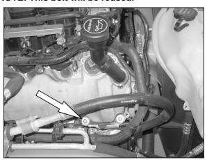
14. Remove the valve cover mounting bolt shown. **NOTE: This bolt will be reused.**
