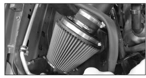
33. Install the air filter assembly onto the K&N intake tube and secure with the provided hose clamp.
