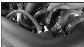
30. Install the supplied brake booster vent hose onto the factory fitting and then connect the other end to the npt fitting in the K&N® intake tube.
