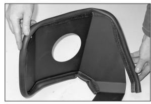
17. Install the supplied edge trim onto the heat shield as shown.
