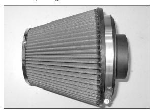
31. Install the filter adapter into the K&N® air filter as shown and secure with the provided hose clamp.
