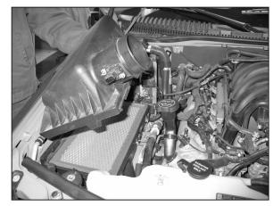
7. Unlatch the three air box lid latches and then remove the lid from the vehicle
