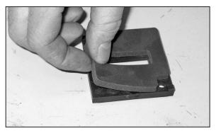
24. Install the supplied gasket onto the mass air sensor adapter as shown.
