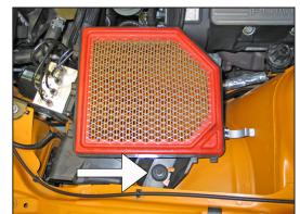
2. Depress the locking tab and then unhook the mass air sensor electrical connection.
