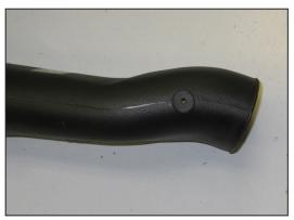
12. Install the supplied  $\frac{1}{4}$ "id vent grommet into the K&N<sup>®</sup> intake tube as shown.
