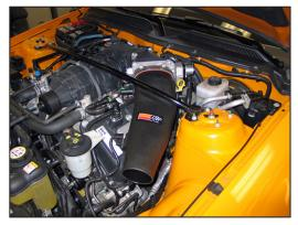
20. Install the K&N<sup>®</sup> intake tube into the throttle body and align with the mounting bracket, then secure with the provided hose clamp and hardware.
