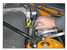
4. Disconnect the vacuum vent line as shown.
