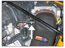
26. Attach the crankcase vent hose to the factory fitting that was installed in the  $K\&N^{\odot}$  intake tube in step #15.
