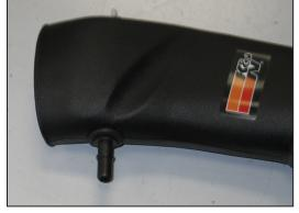
16. Install the factory crankcase vent fitting into the grommet installed into the K&N tube in step #14.
