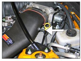
25. Connect the vacuum vent line onto the ¼" hose mender that was inserted in the K&N<sup>®</sup> intake tube during step #13.
