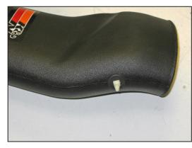
13. Insert the supplied 1/4" hose mender into the grommet that was installed in the previous step.
