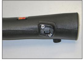
11. Install the mass air sensor into the K&N $^{\odot}$  intake tube and secure with the provided spacers and m4 bolts.
