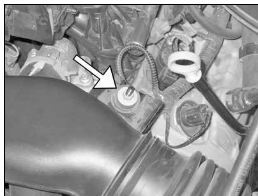
4. Remove the nut which secures the stock intake tube to the mounting stud.
