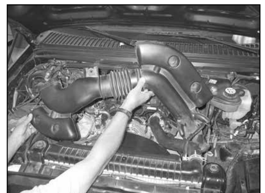
5. Unhook the factory fresh air tube from stock air box and radiator core support. Then remove the fresh air tube from the vehicle.
