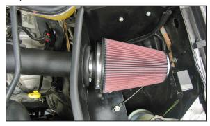
32. Install the air filter assembly onto the K&N<sup>®</sup> intake tube and secure with the provided hose clamp.
