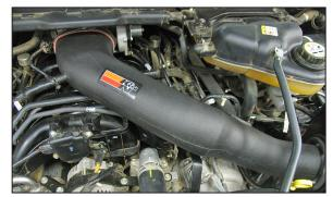
26. Install the K&N<sup>®</sup> intake tube onto the throttle body and align the mounting bracket so that it sits on the 8mm stud protruding from the cylinder head.
