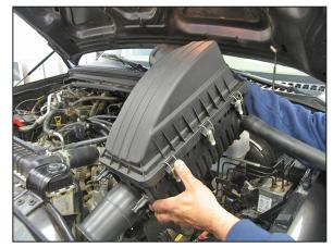
6. Pull up on the rear of the air box assembly to dislodge it from the mounting grommets and then remove the air box from the vehicle. NOTE: K&N recommends that customers do not discard factory air intake.
