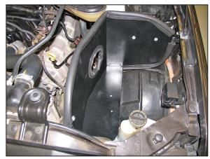
20. Install the heat shield assembly into engine compartment as shown.
