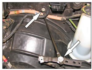
8. Remove the two bolts, which secure the support rod to the inner fender and to the core support, then remove the support rod from the vehicle. **NOTE: Do not discard the support rods and bolts, as they will be reused.**
