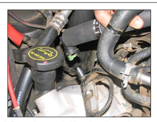
3. Rotate the green locking tab on the crank case vent connector at the valve cover counter
