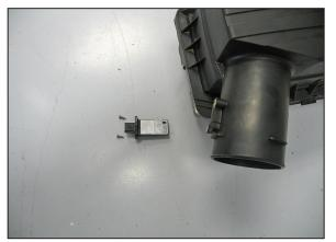
11. Remove the two mass air sensor mounting screws with the T20 TORX wrench provided and then remove the sensor from the air box as shown.
