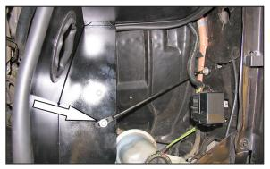
23. Reinstall the support rod with the factory mounting bolts removed in step #8 as shown.
