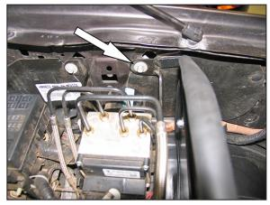
21. Place the rear heat shield bracket between the inner fender and the ABS pump mounting bracket and secure with the factory mounting bolt removed in step #9.
