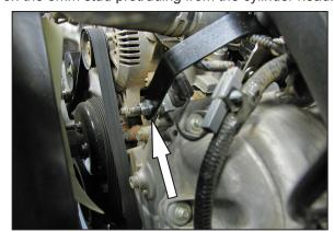
27. Secure the tube mounting bracket to the 8mm stud with the nut and washer provided. Align the K&N<sup>®</sup> intake tube for best fit and then tighten the hose clamp and bracket mounting hardware.
