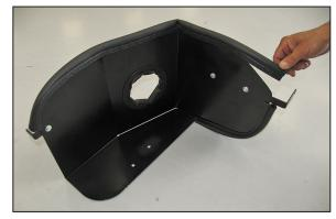
19. Install the edge trim to the heat shield as shown.
