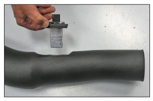
14. Install the mass air sensor assembly into the K&N<sup>®</sup> intake tube as shown with the opening pointed towards the filter end of the tube.
