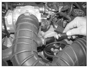
3. Release the locking ring and then disconnect the crank case vent tube.
