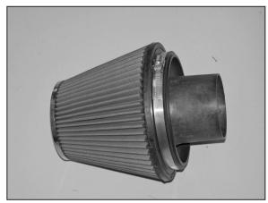
20. Install the air filter onto the filter adapter and secure with the provided hose clamp as shown. NOTE: Drycharger<sup>®</sup> air filter wrap; part #
