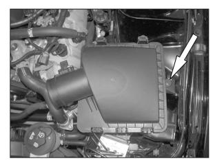
5. Remove the airbox mounting bolt shown.
