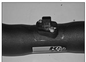
15. Install the mass air sensor into the K&N® intake
