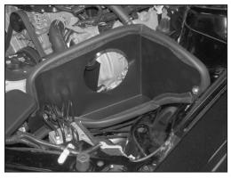
15. Install the heat shield and secure with the provided hardware as shown.
