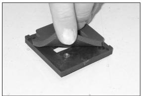
17. Install the provided gasket to the back of the K&N<sup>®</sup> mass air sensor adaptor plate as shown.
