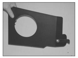
12. Install the "L" bracket (07158) onto the front of the heat shield as shown with the provided hard-ware.
