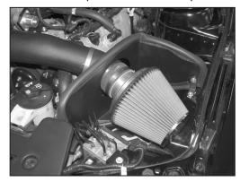
25. Install the air filter assembly onto the K&N<sup>®</sup> intake tube as shown and secure with the provided hose clamp.
