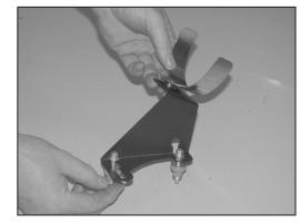
9. Install the valve cover bolts removed in step #8 into the tube mounting bracket as shown passing through the key hole portion and then slide the bolts to the end of the slots.
