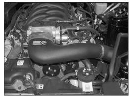
19. Install the K&N<sup>®</sup> intake tube into the silicone hose at the throttle body and onto the saddle bracket assembly then secure with the provided hose clamps as shown.
