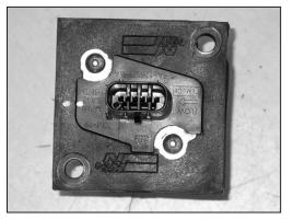
17a. Install the mass air sensor into the K&N<sup>®</sup> mass air sensor adaptor and secure with the provided hardware.
