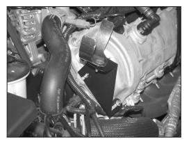
10. Install the tube-mounting bracket onto the valve cover as shown and secure with the stock hard-ware removed in step #8.
