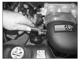
20. Install the supplied vent hose onto the vent port on the valve cover and then onto the K&N<sup>®</sup> intake tube as shown.
